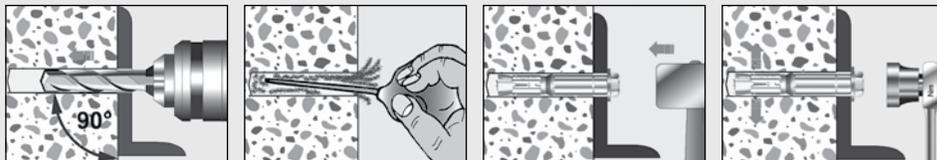
3 Assemble the nut & washer past the impact end of the SRS+. Use a hammer to tap the anchor through the part being fastened into the drilled hole until the washer is in contact with the part.
