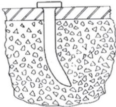
"Fish-hooking" can occur when a partially driven fastener hits a hard object, which bends and deflects the shank. "Fish-hooking" may reduce holding power, usually increases spalling and can be a potential hazard from an escaping fastener and/or particles of masonry. Always use a shield or fixture on the tool unless the item fastened provides equal or greater protection - especially when driving threaded studs or eye pins directly into masonry.
