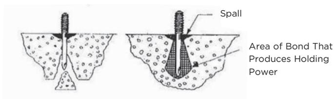
As a general rule, when fastening into average concrete, the fastener should penetrate 7 to 8 times the shank diameter. In hard concrete, 5 to 6 times the shank diameter's penetration would normally be sufficient for proper holding power. In soft concrete, 9 to 10 times the shank diameter would be appropriate.
